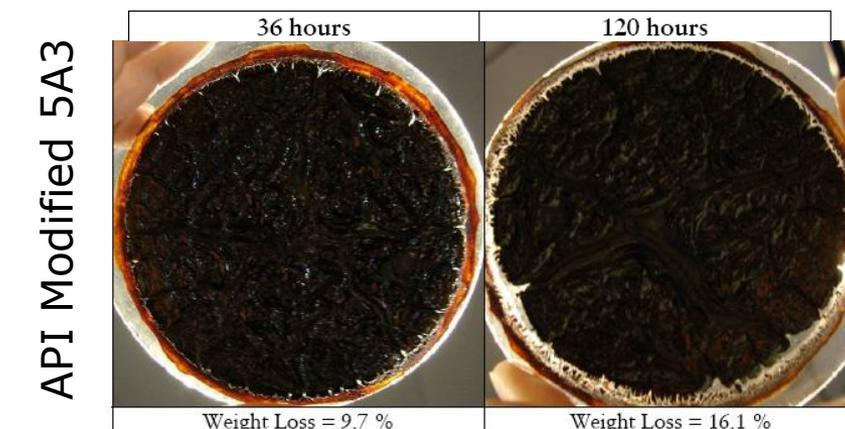
Figure 1. Thread compounds after exposure to 180°C.
